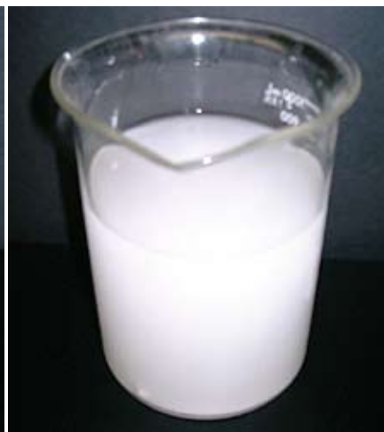
Left: Water at the correct pH dissolves the materials to form a clear solution. Right: When a calcium product is added to high pH water, a cloudy, insoluble precipitate forms.
